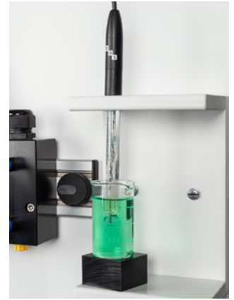
Maintenance station at the YSI Water Monitoring Panel
